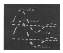
Oscillograms of current (top) and voltage (bottom) during a discharge with a voltage (at the condenser) of 4800 V, abolishing auricular fibrillation in patient B. Amplitude of voltage (1st half-wave) at the patient 940 V, amplitude of current 26 A. Time marker (between beginnings of adjacent dashes) 1.6 msec.
